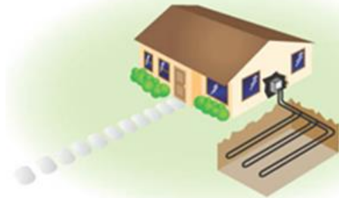
Closed Loop Horizontal Systems
